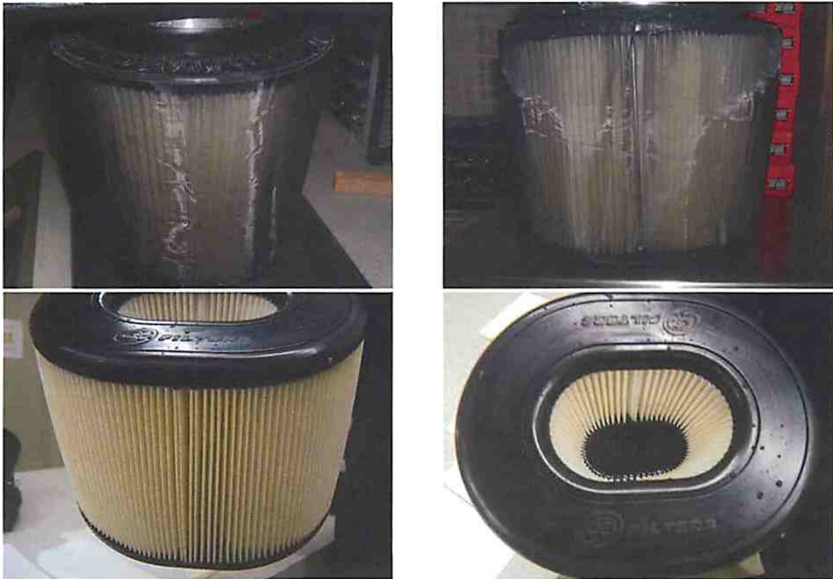
Figure 6. Some General Photographs during and after Testing (Run 4; Unit with Wrapped Disposable Filter + Wrap Material on Outlet of Lower Scoop Section) (Continued)
