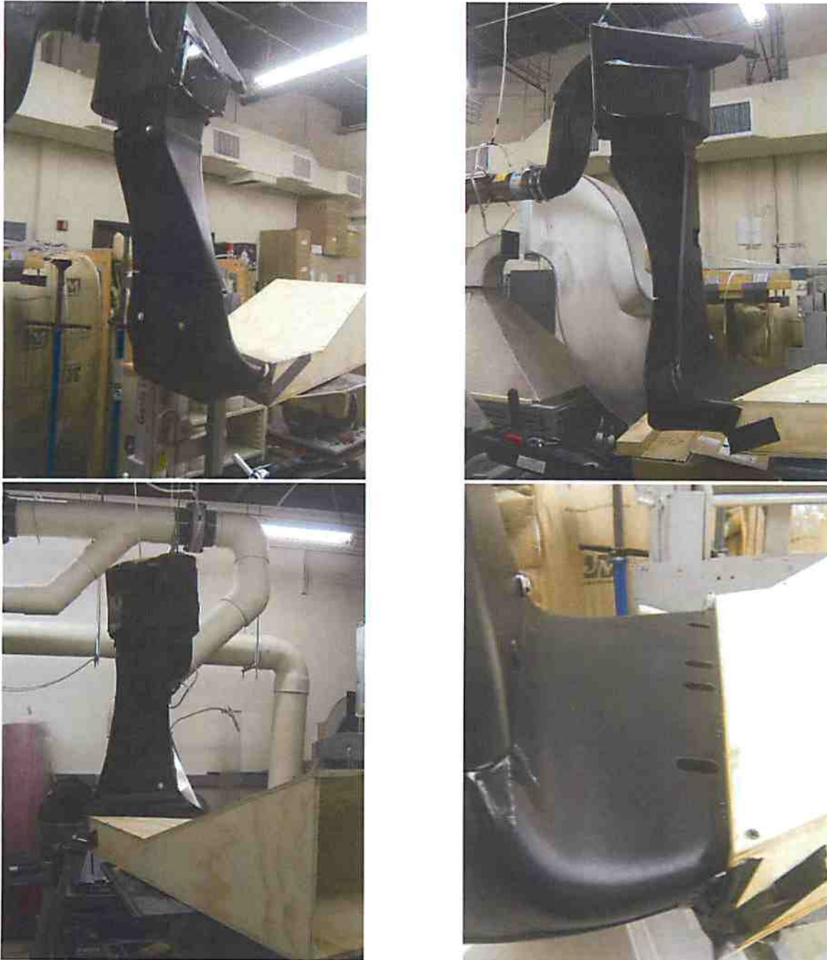
Figure 1. General Test Arrangement (spray wand moved back and forth across scoop inlet) [Bottom 2 rows show wrap material applied to outlet of lower scoop section]
