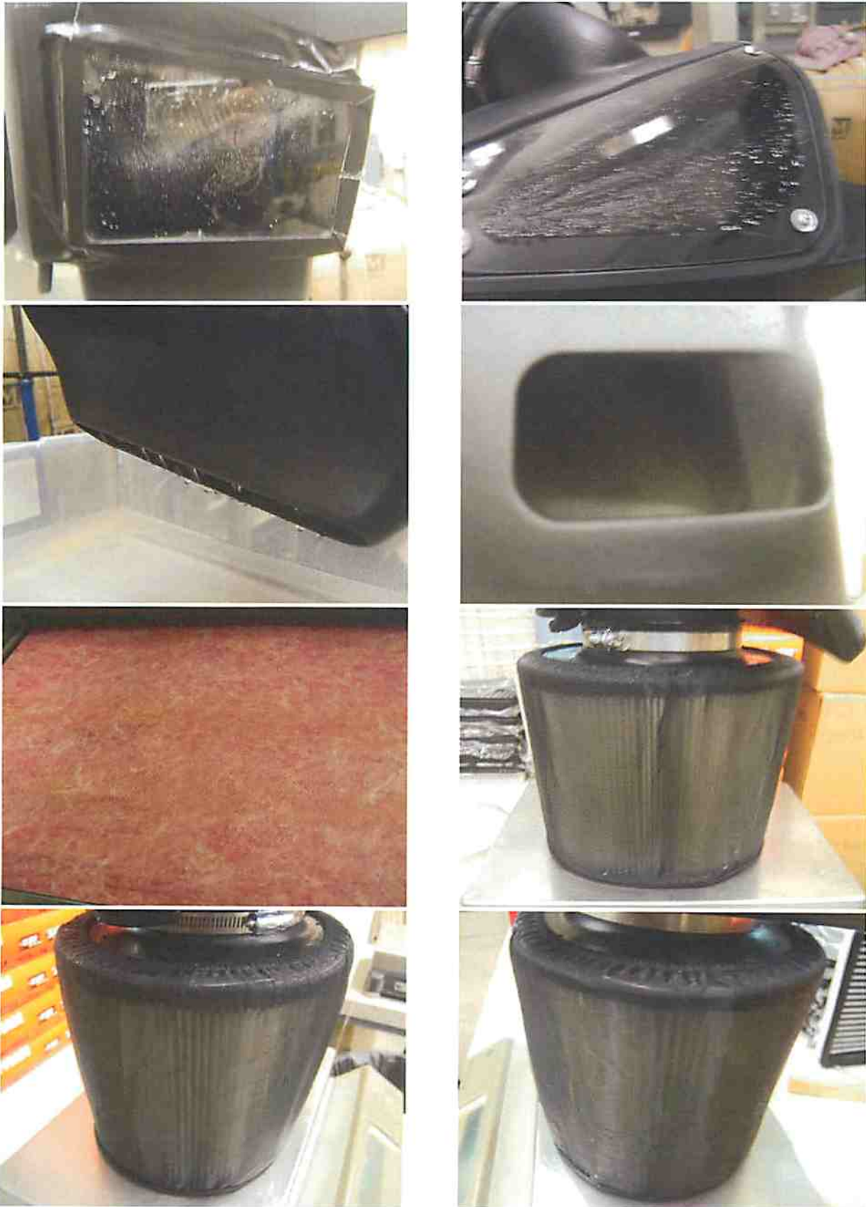
Figure 6. Some General Photographs during and after Testing (Run 4; Unit with Wrapped Disposable Filter + Wrap Material on Outlet of Lower Scoop Section)
