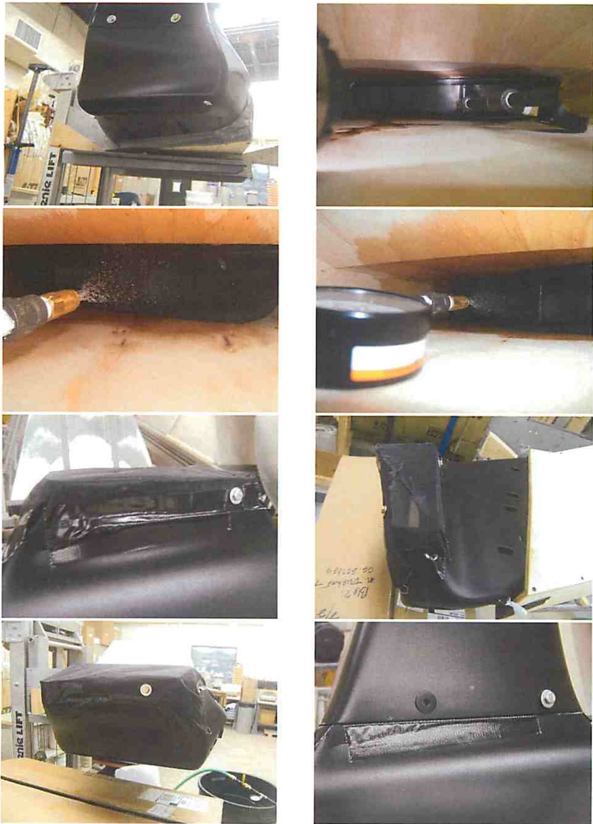
Figure 1. General Test Arrangement (spray wand moved back and forth across scoop inlet) [Bottom 2 rows show wrap material applied to outlet of lower scoop section] (Continued)
