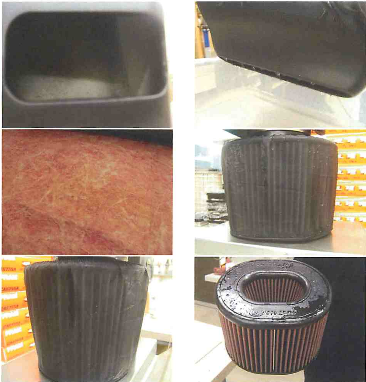
Figure 5. Some General Photographs during and after Testing (Run 3; Unit with Wrapped Cotton Filter + Wrap Material on Outlet of Lower Scoop Section) (Continued)
