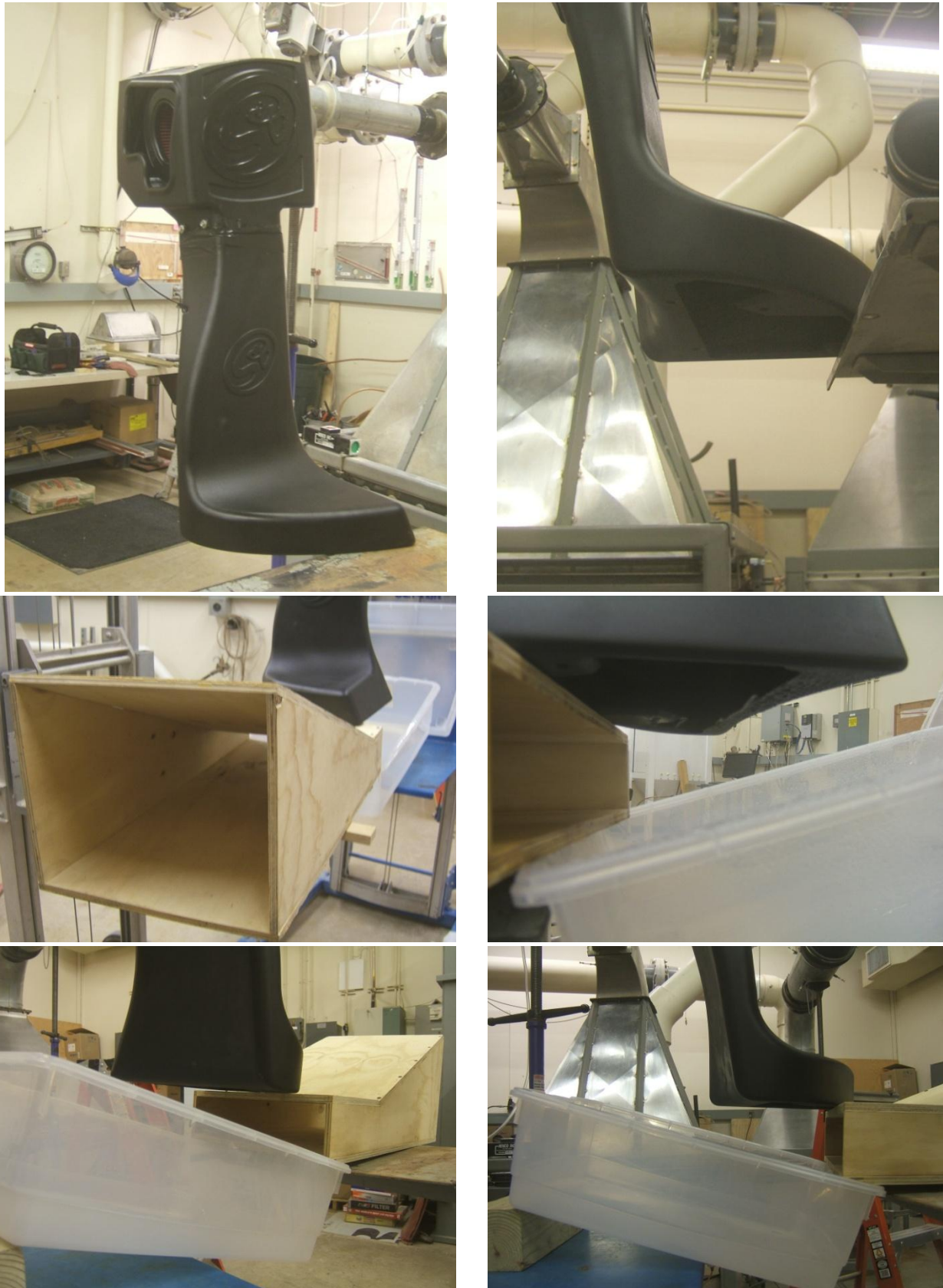
Figure 2. General Test Arrangement for 75-5058 Intake with AS-1001 Scoop (top row: airflow testing; other rows: water spray testing)
