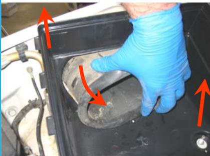
7. Attach the S&B Filter Adapter (I) to the S&B Air box (H) while slipping the air filter over the flange at the same time.
