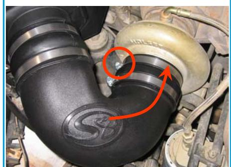
4. Place a rubber spacer (R) over each of the factory studs on the inner fender, then set the S&B air box (H) in place over the studs.
