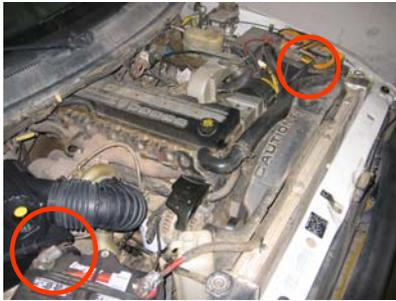
5. Determine whether your vehicle has SAE or Metric threaded studs and use the appropriate 1/4-20(F) or M6(L) lock nuts supplied and fender washers to secure the S&B air box (H) to the inner fender.
