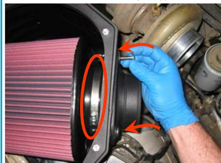
12. Slide the S&B Hump Adapter (Q) over the filter adapter (I), center over the gap between the tubes and secure the #72 Hose Clamps (K).
