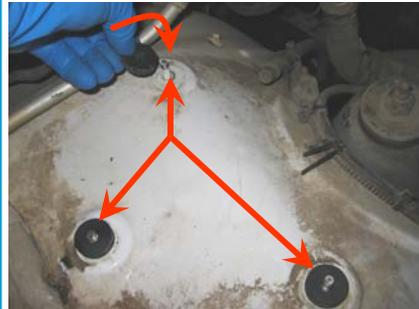
8. Secure the adapter using the 5/16 screws (J) provided. Then tighten the # 80 hose clamp to secure the filter to the adapter (I).
