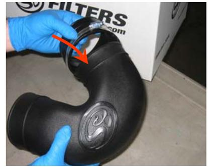
2. Loosen the hose clamp at the turbo inlet, then unclip the air box top and remove the OE intake tube and air filter.
