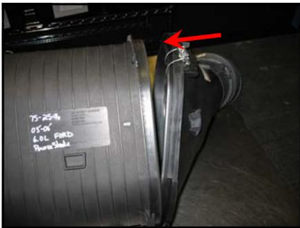
14. Reinstall the intake assembly into the vehicle and secure the prongs on the filter housing into the appropriate grommets.
