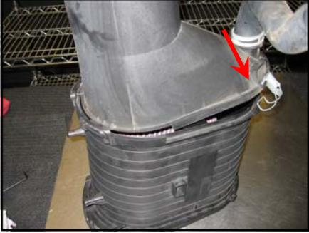
13. Reinstall the intake tube to the filter housing assembly and secure using the clamps.
