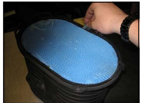
9. Remove the filter from the housing by pushing it out from the opposing side.
