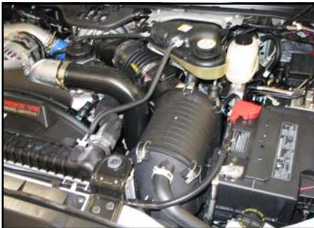
2. Disconnect the radiator overflow. Make sure the system is cold. The tube is under pressure.
