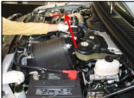
6. b) Remove the complete intake assembly from the vehicle.
