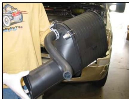
7. Isolate the filter core from the OEM intake tube and OEM snorkel by unclipping the clasps.
