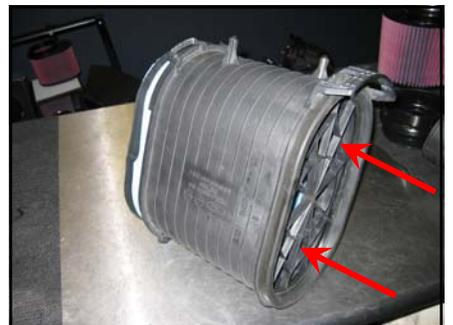
10. Install the S&B High Performance Filter into the open end of housing as shown. The fit is very tight. Use a small amount of soapy water to aid in installation if necessary.
