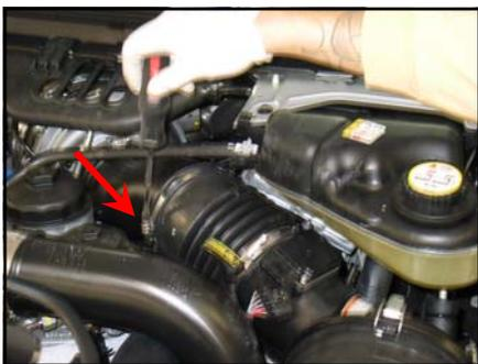
16. Reinstall the radiator overflow line.
