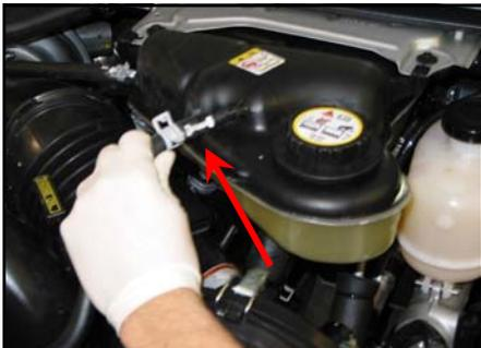
3. Disconnect the electrical connection for the air filter gauge.
