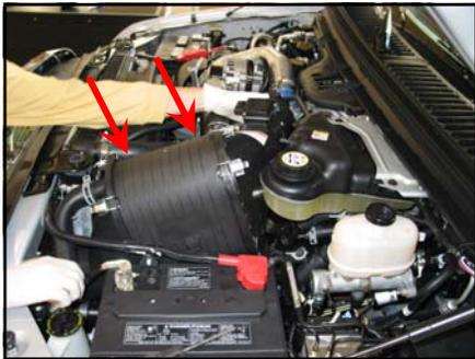
15. Tighten the hose clamp at the turbo manifold. Reconnect the electrical connections for the MAF sensor and the Air Restriction gauge.
