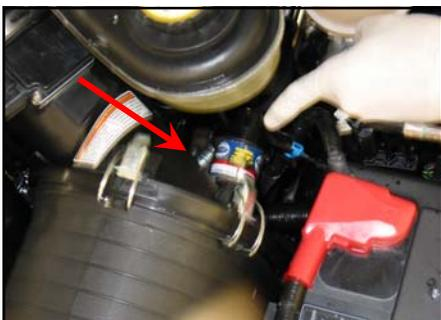
4. Disconnect the electrical connection to the Mass air flow sensor OEM air intake tube and remove the tube. Disconnect the Mass air sensor and remove the sensor from the OEM air box.
